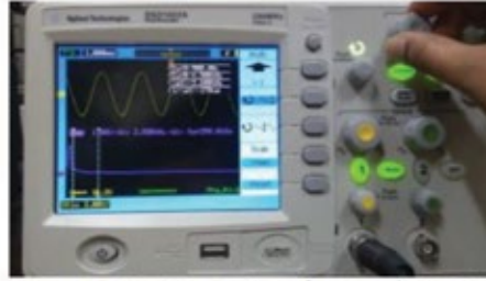
Viewing Fast Fourier Transform on the DSO
