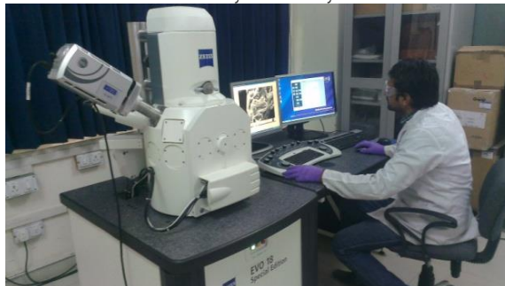
Scanning Electron Microscope and Electron Dispersion Spectrometer
