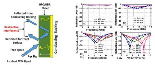
Attenuation mechanism in BFO/NBR composite in the microwave range (left panel) and reflection Loss (R.L.) over frequency range 2–12.4 GHz and matching thicknesses of different ferrite loaded rubber composites (right panel),
