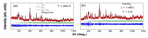
Neutron diffraction measurements (a) 300 K and 3 K on bulk FeVO<sub>4</sub> powder sample Outcome: Highly anisotropic nature of FeVO4 is demonstrated with large variation in different lattice parameters with temperature.
