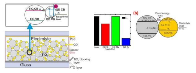
QDSSC structure with respective band diagram (left panel), and TM doping strategies in QDs for efficient PV response.
