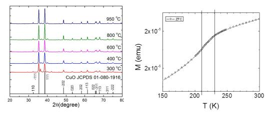
XRD patterns of CuO nanoparticles and representative ZFC curve shoing the respective AFM transitions.
