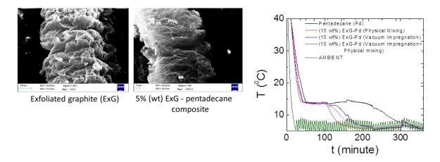
Exfoliated graphite as a host matrix(left panel, left figure), with PCM (left panel right figure) and T-history meausrement data on developed composites.
