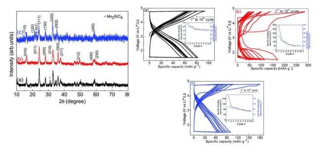
XRD patterns and respective charge/discharge capacity of LMSO system
