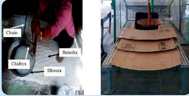
Figures 11 (a) and (b): Traditional method of making Batasha; and Improved structure for making Batasha
