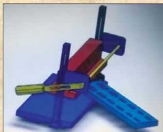
Figure 5(a): CAD model of manual Bhilawa decortication machine
