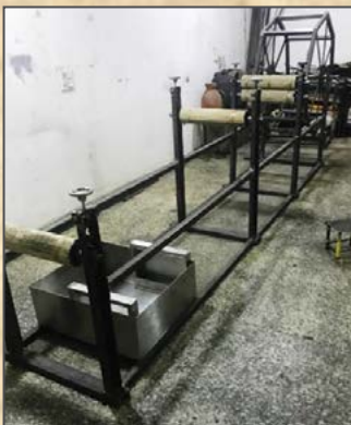
Figure 7(b): Actual Model of the new Drive Mechanism/ Street sizing machine
